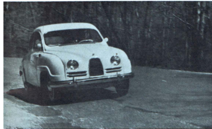
The SAAB cruises through a bend, which is slightly cambered, at 50 mph. Optics create illusion of steeply banked road. Accelerating through turns, car was absolutely unswerving, but when braking in turns, loss of control was evident.
