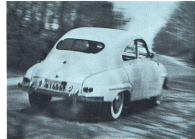
The SAAB cruises through a bend, which is slightly cambered, at 50 mph. Optics create illusion of steeply banked road. Accelerating through turns, car was absolutely unswerving, but when braking in turns, loss of control was evident.
