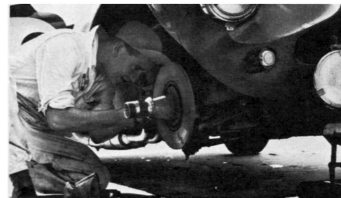
Spot brakes on DB3S get 2½ minute change at Sebring during race. The pie-slice could be removed and replaced quickly during fuel stops.
