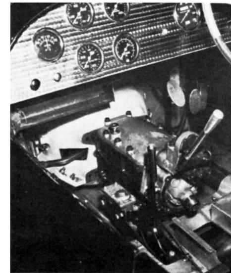
Jag box is mounted to engine by special adaptor. Note emergency brake system. Main brake system is alongside engine on right side. Master cylinder is from Chevrolet truck.
