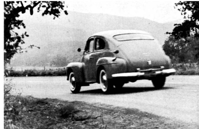
Taking leave of the curve, the 444's attitude has understeer effect, tail out, nose into turn. With a back seat passenger or some trunk luggage, 50/50 distribution can be hit on nose.
