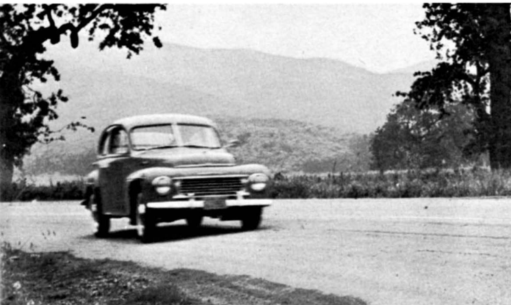
Entering SCI test curve at 50 mph, car rode flat and steady. Some lean can be detected, however, in photo. Good cornering comes from its almost equal weight distribution, with 2 aboard.
