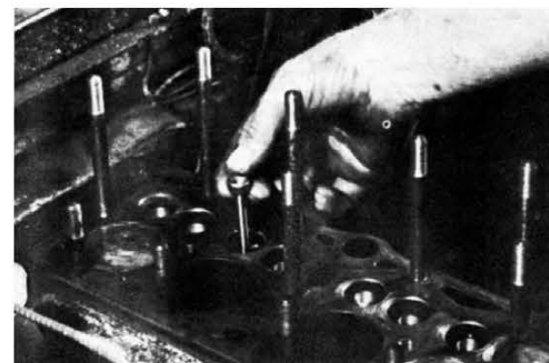
1 The eight inter-tappets from the kit are oiled and inserted through the old valve guide holes. This is done only after block is cleaned and studs set in.
