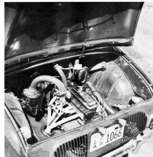
Hanging from the light alloy cylinder head the bunch of bananas exhaust converges directly into muffler beneath belly pan. Note accessibility of engine.
