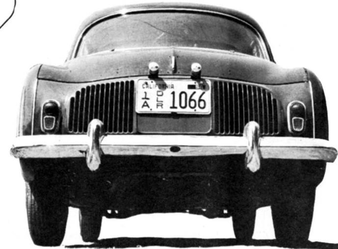
Telltale louvers in the rear just above bumpers are the only indication that the Dauphine is a rear engined vehicle.
