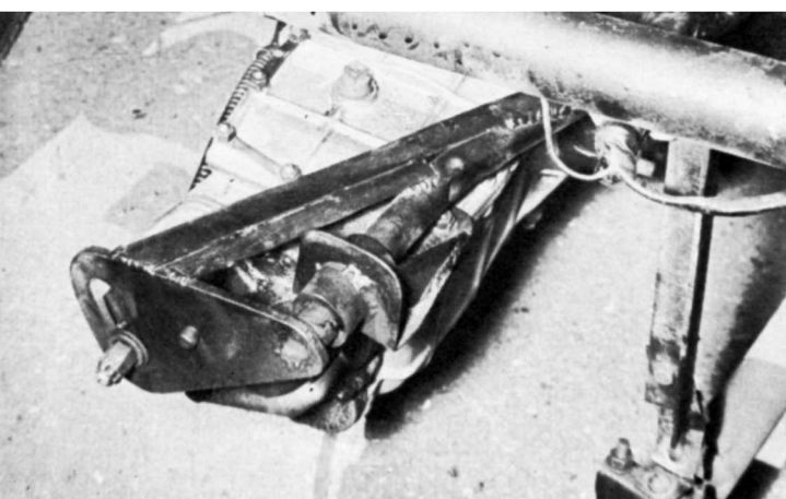
Rear view of scotch yoke. Bar part of yoke connects to stick shift at front. Slotted plate moves up and down, in and out, operating bell crank.
