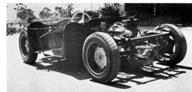
This rear view shows the high kick-up in the rear needed for new engine hanger built by Chuck Clemens. Engine is reversed, set ahead of axle to improve weight distribution.
