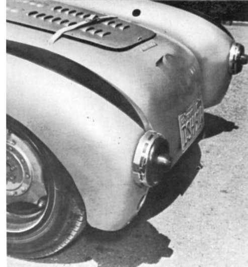
The engine hatch was cut into the body after the mold was completed. Lowered cover is aluminum. Rear lanterns are '53 Ford tail lights.
