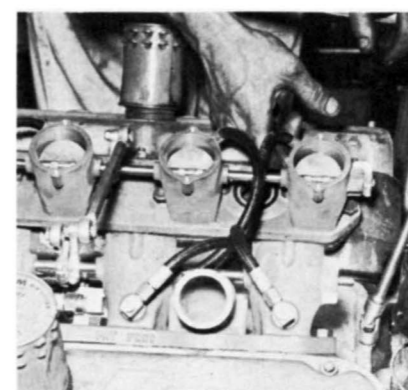
5 Idle mixture and speeds are set at factory, require little adjustment. Idle is adjustable by turning locknut on throttle screw.
