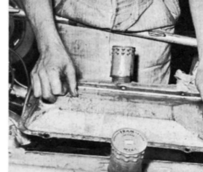
2 Stock valley cover can be sent to kit maker, or a new plate with junction block can be had. Junction block must be installed at factory.
