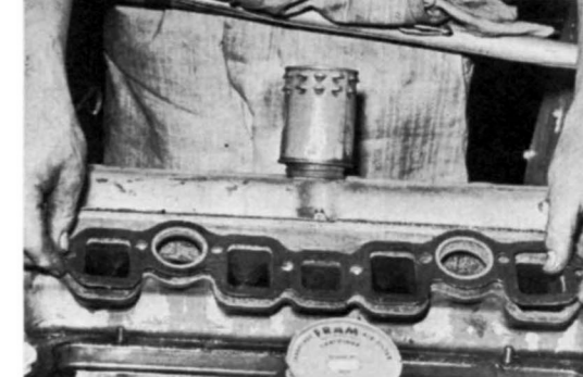
3 A new thin gasket is installed to replace gaskets which were removed. Thicker stock gaskets may cause throttles to stick when opened.
