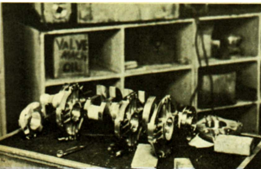
Crankshaft and webs. These webs bolt to crankcase bulkhead giving 360 degree support to bearings.
