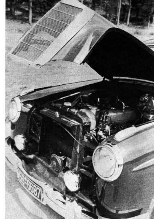
Grille lifts neatly away with the hood. The 112 bhp engine comes equipped with dual Solex downdraft carbs.
