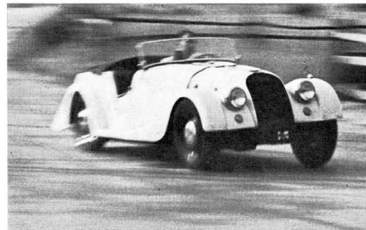
Stiff springing keeps Morgan clinging fast, and flat, through tight bends. This factor coupled with the car's excellent acceleration, makes it a tough customer on short courses.
