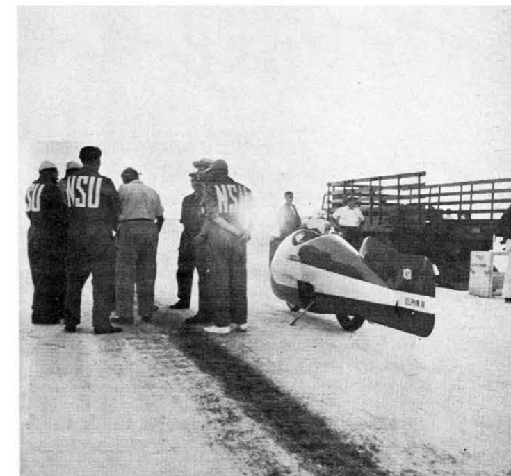
Wind velocity had to be zero over entire course area. Unfortunate fin-over-canopy flip occurred when Herz tried to correct error in course direction caused by side wind.
