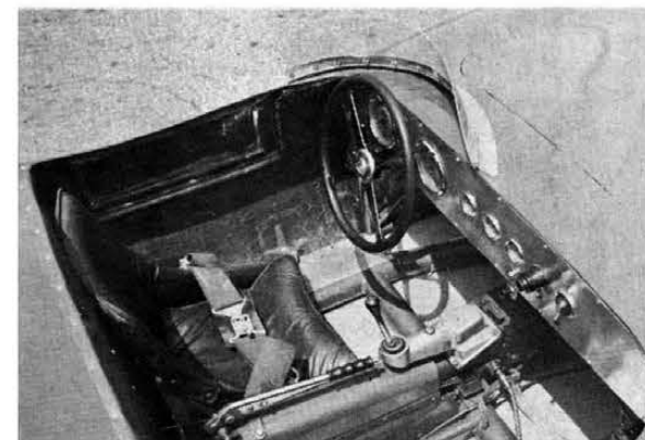
Cockpit layout is designed more for utility than for comfort. Instruments are placed for easy reading. Note wide seat belt for maximum safety.
