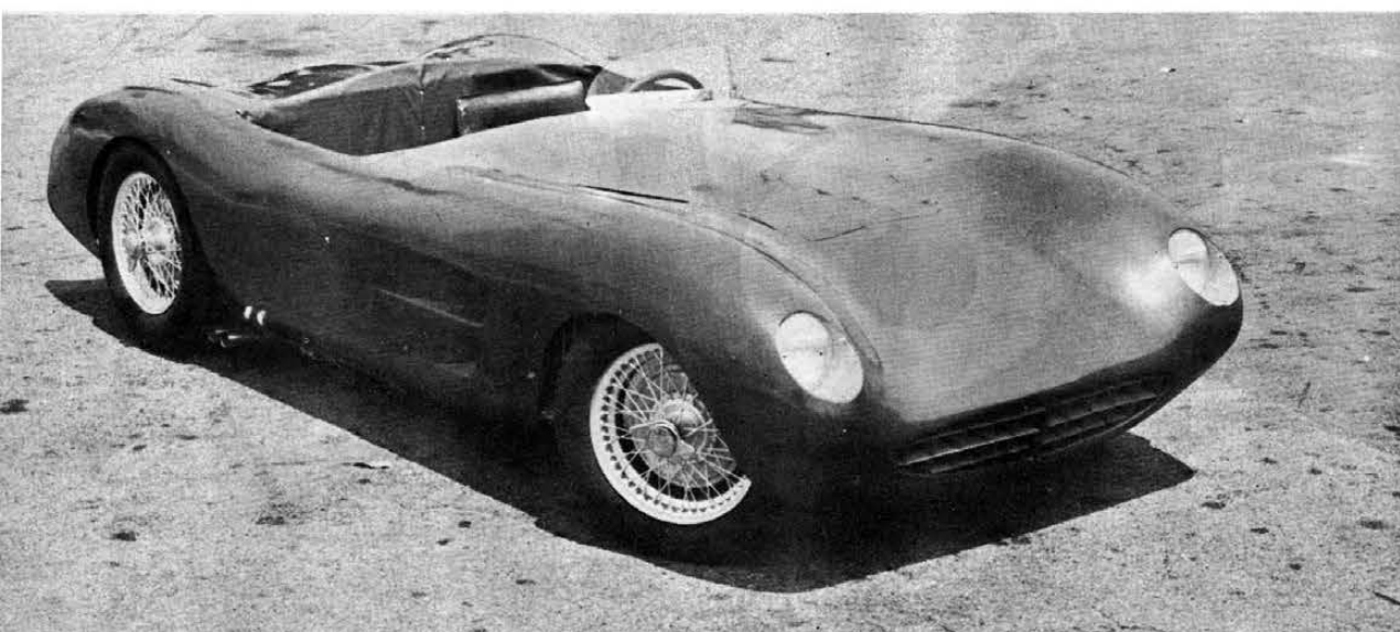
Dressed in its attractive plastic shell, which weighs only 75 pounds, the PMG Mistral sits 4½ inches from the ground. The reinforced body has its color laminated into it at the time of manufacture.
