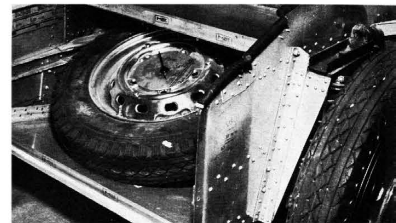
Angle bars, and U-shaped channel members add to the stiffness of the sheet aluminum frame. All joints are riveted. Spare tire is carried in pocket at rear.
