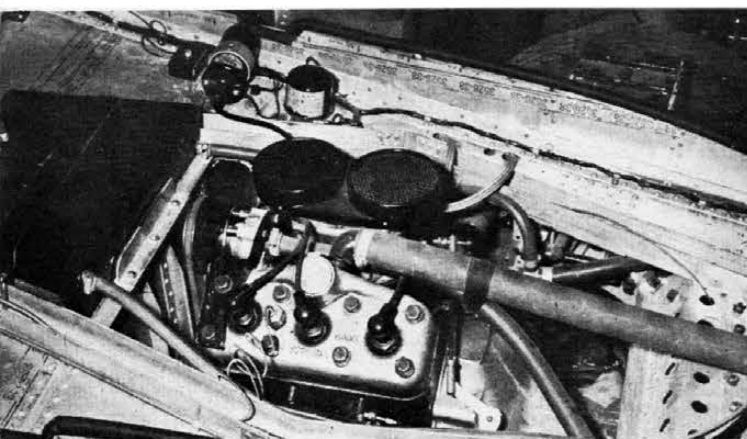
The three in-line cylinders of the two-stroke engine are corked by a light alloy head with a modified water outlet. Radiator is placed at rear of mill, header tank fore.
