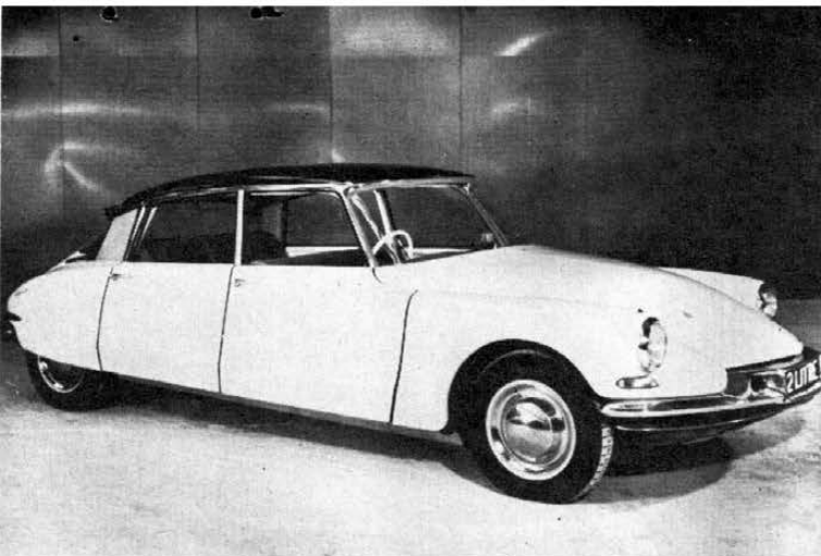
The DS 19 Citroën manages a full turn in 36 feet despite its 123 inch wheelbase.
