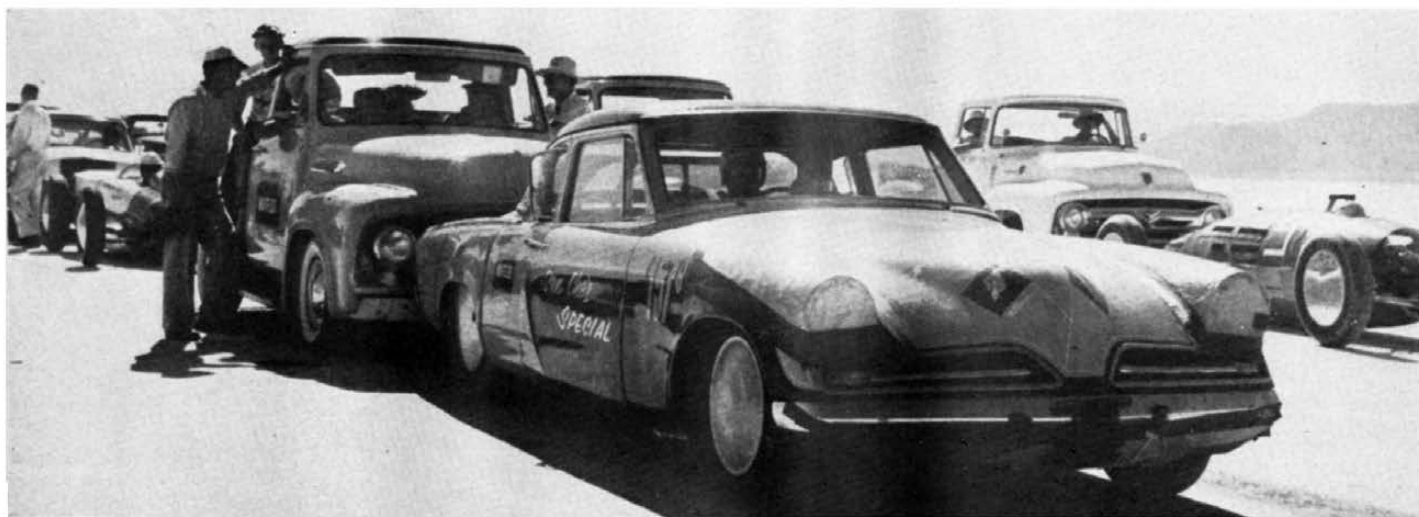
The San Chez-Cagle-LeMion '53 Stude with Chrysler plant. Before piston seized, the car turned 185.18 one way on 95 percent nitro and 5 percent benzole. Note driver's position is in middle of car.
