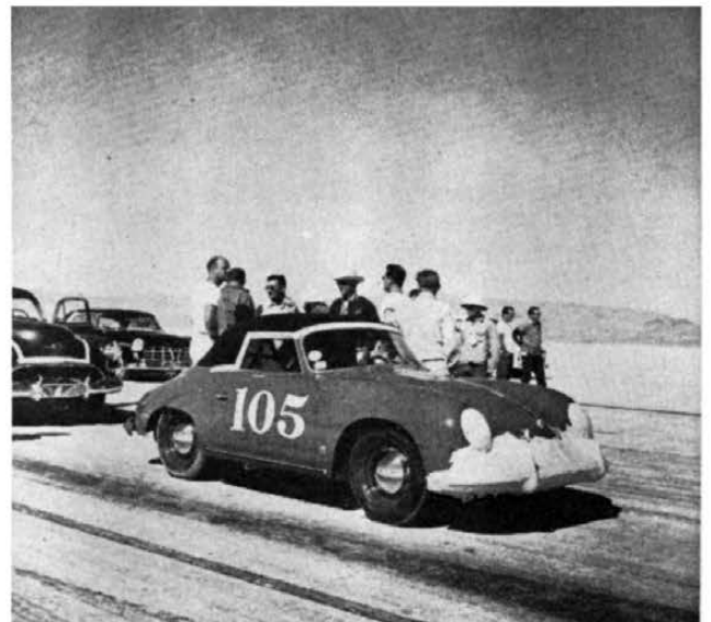
Based on an Allard chassis, Lavell's car alternated two De Soto Adventurer engines—one with 341 and one with 357 cu. ins., and torque converter transmissions. Car walked through traps.
