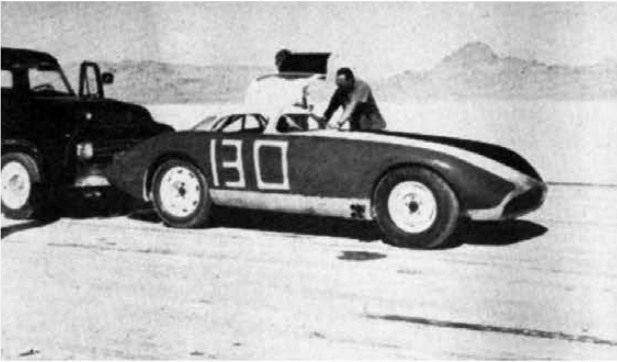
The Barnes-Larsen car. Engine was built by Ray Brown, and turned 350 bhp on gas. Car's body was constructed by Robert Sorrell. The car weighs 1600 lbs. and carries an Allard de Dion rear.
