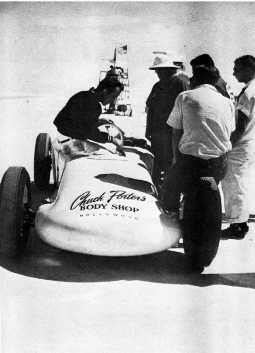
Chuck Porter built odd looking nose for '27 T roadster belonging to T. Ruddy and M. Weinstein. Theory of front is that needle nose or wedge leaves too much room for turbulence between body and wheels. Theory worked—200.009.
