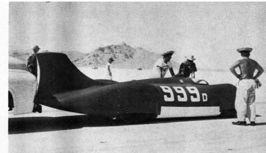
The Herda-Cramer streamliner gets final check before run. Bolts in blower drive sheared several times. Overheating caused car to fail.
