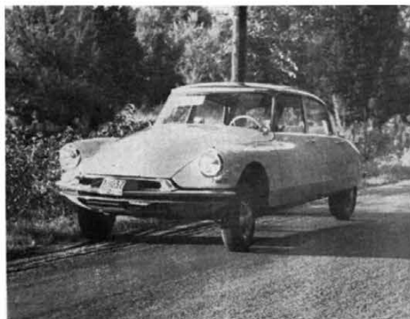
Road clearance of the DS 19 adjusts from within driver's compartment. Here car sits at 13 inches.
