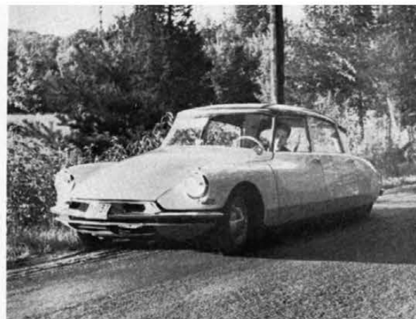
By exhausting the hydraulic fluid from suspension cylinders, Citroën is placed just 3 inches above road.
