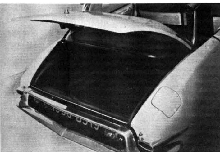
With the spare wheel conveniently carried in the front, and the fuel tank rectangular in shape and pushed well forward, the trunk space becomes unusually deep.
