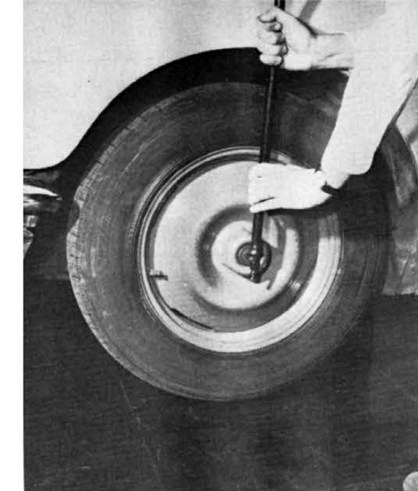
Allen type nut holds driving wheels on hexagonal drive-key. Remove with a specially supplied wrench.
