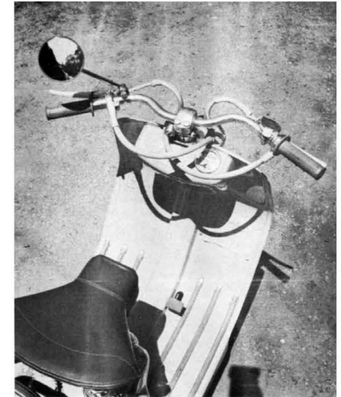
Driver's view of the Lambretta shows the lack of instruments except for speedometer and odometer.
