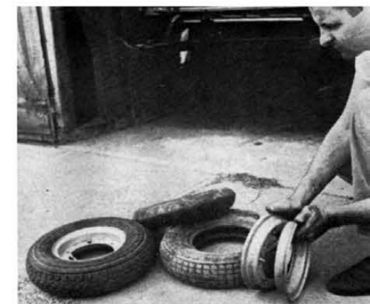
Change of tires is easily accomplished due to split rim wheel which requires only the wrench supplied with bike.
