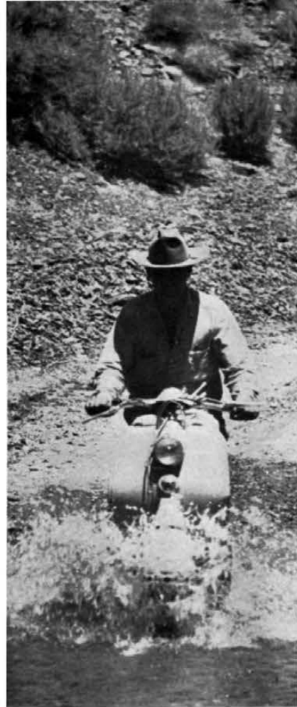
The watercourse at Silver Canyon had to be forded many times during trip. To find limit, SGI's chief tester made 10 passes before ignition quit.
