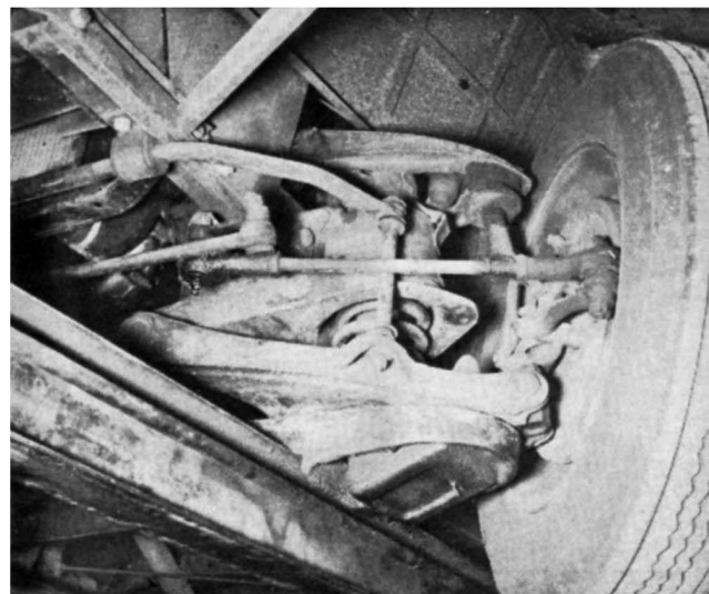
Front running detail. Anti-roll torsion bar is 3/4 inch in diameter. Note massiveness of wishbones for such a light car.
