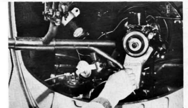
Unhook stock throttle linkage. Remove oil bath air cleaner from Solex carburetor, but leave carb in place. Lift out the manifold (and heat riser) along with the Solex.
