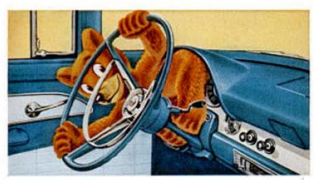
This Lifeguard steering wheel has a new deep-center construction to reduce the possibility of driver being thrown hard against the steering post in case of an accident. Our Ford engineers have mounted the rim of the wheel high above the recessed steering post to help "cushion" your chest against severe injuries from impact.
