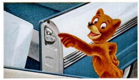
You're twice as safe if you stay inside the car in an accident. Statistics prove it conclusively. So our Ford engineers have designed these new Lifeguard door latches with a *double grip* to reduce the possibility of doors springing open in a collision.
