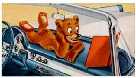
Optional Lifeguard padding protects you against accident injuries by providing a "crash cushion" on both the instrument panel and sun visors. It is five times more shock absorbent than foam rubber. New Lifeguard double-swivel rearview mirror that "gives" on impact and resists shattering is standard on all '56 Ford models.
