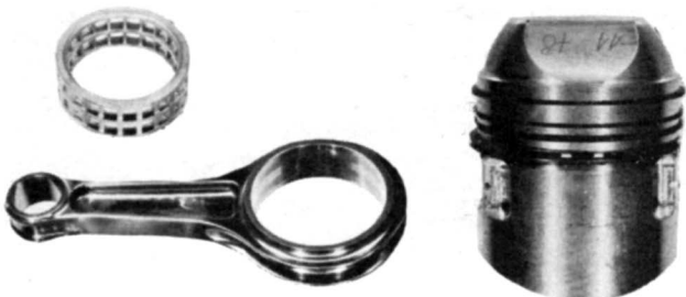
Alloy cage locates rollers, which run direct on surface of crank and rod big-end. Construction of rod needs little comment. Very slight valve cutouts are needed on piston dome.
