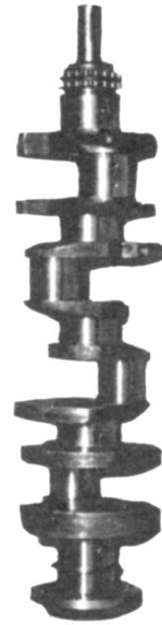
Five-bearing crank is husky forging, ample journal overlap. Counterweights are big, drilled for balance. Sprocket is for roller timing chain.
