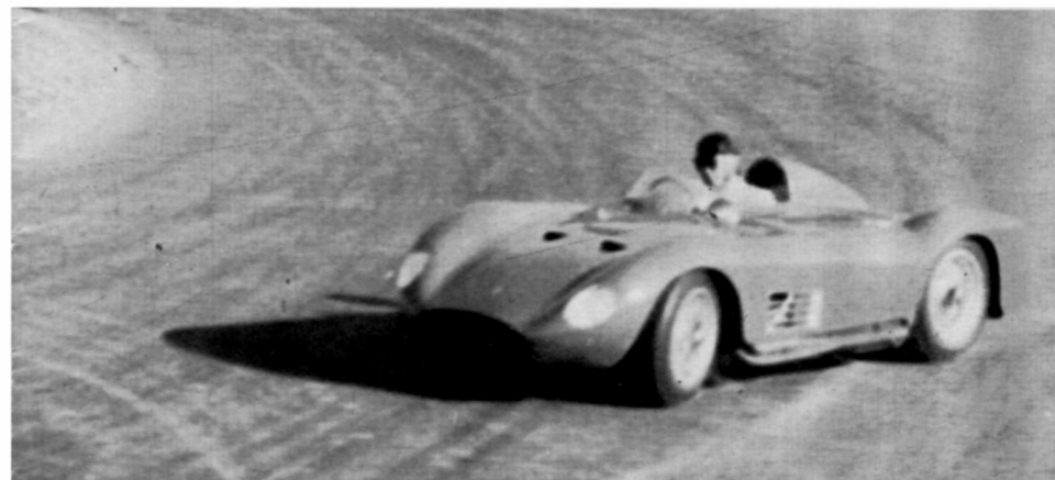
Pollack puts 200 SI stability to the test, finds balance and handling in top class. Slide here was readily provoked by stab at throttle. Maser understeers, and if taken too far this can bring it back into line.
