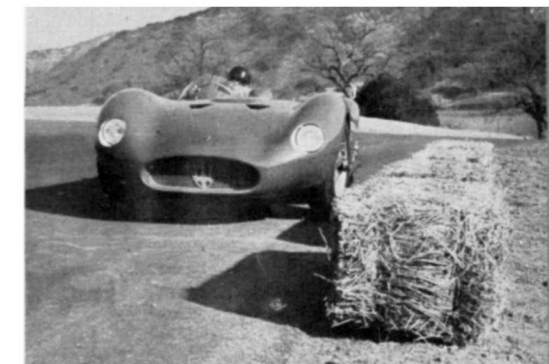
Latest Maserati bodies are clean, Lotus-inspired, have longer nose for better penetration and lower duct diffusion angle.
