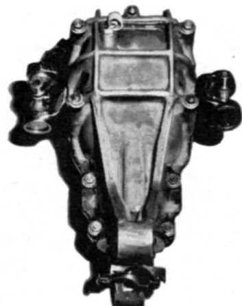
Axle case is rough cast, has breather at top. Four bearings hold pinion, and drive is through ZF differential.
