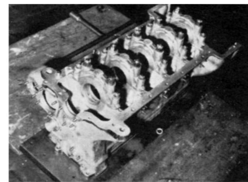
Crankcase and sump separate at crank centerline, lateral strength being provided by four-bolt caps, wide webbing.
