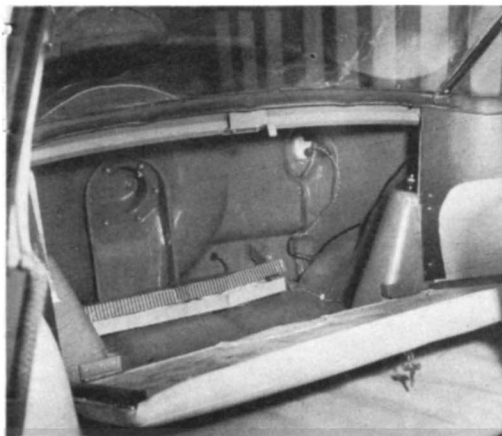
Trunk is reached through rear seat backrest only. Space is at premium, but small parcels can be accommodated in the back seat or trunk.
