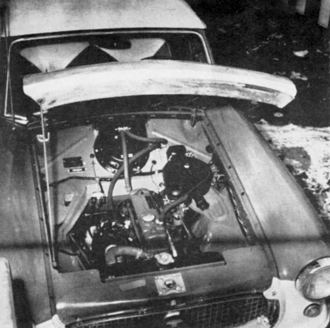
Everything in engine compartment is accessible. Note, that while car is unit-frame constructed, skin is not stressed. Pressed panels offer support.
