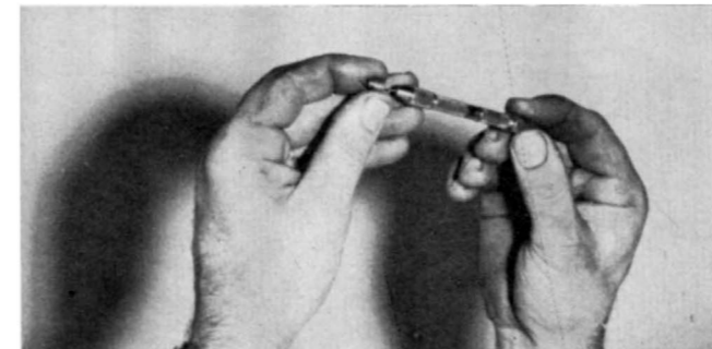
8 Standard drills in proper size were used to enlarge jets. Drill itself is held solidly in a pin vice and the jet is twisted, not drilled. Increases are made in small steps of one drill-size at a time to prevent gouging jets.
