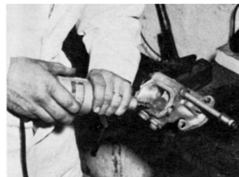
5 Steel wool is used to remove the tool marks made by high speed rotary file in the clean-up process. It also gives the castings a high polish.
