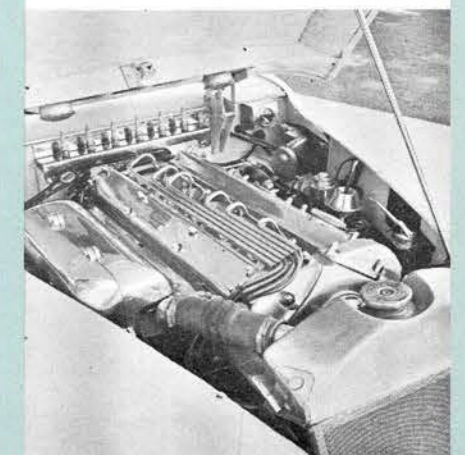
Aluminum pressure box fits over carbs keeping pressure throughout the entire carb layout equal. In compartment are oil can, extinguisher, and extra plugs.
