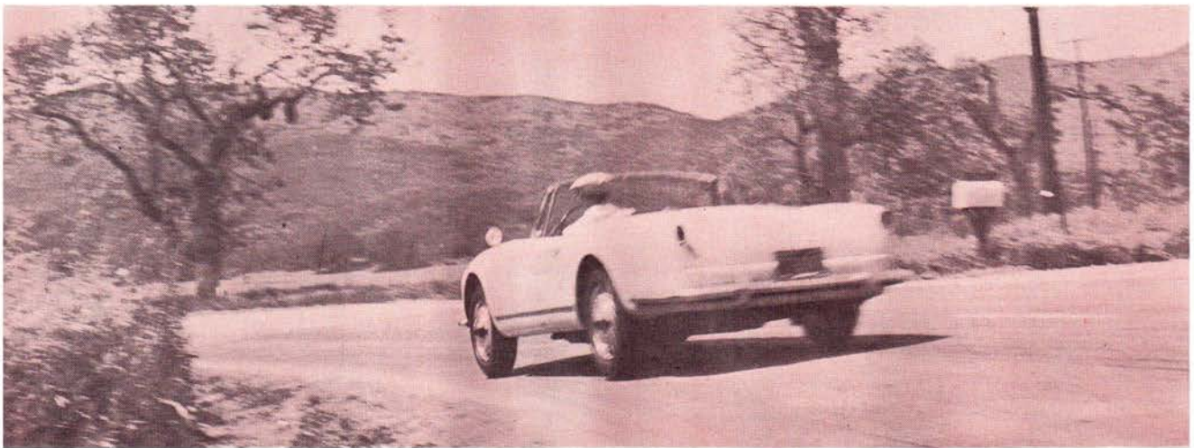
Cornering hard through test bend, Spyder leaves traces of rubber. This "stage three" cornering at speed produces 4 wheel drift.
