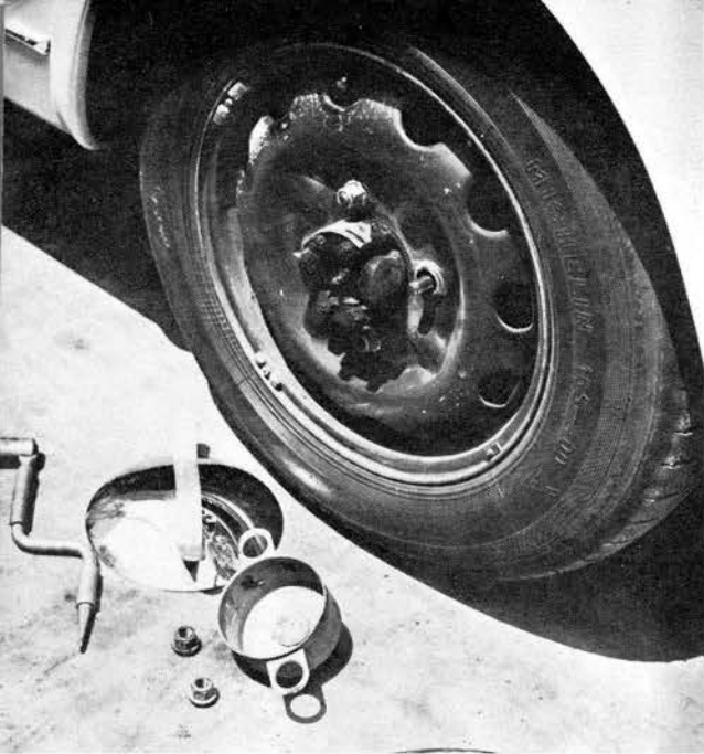
Rear wheel with lug wrench, hub cap and special wrench, and outer U-joint cover which is retained by large nuts. To keep friction losses low, and extend life of joint, Lancia locates external U-joints outside of the wheels. Greater length of half-shafts reduces angular deflections in joints.
