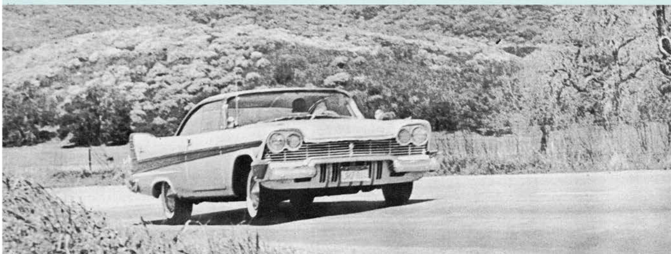
Sharp inward turn of front wheels indicates strong understeer characteristics. At cornering speeds of 55 mph, the rear wheels would slide outward very gradually. Body roll was very slight.
