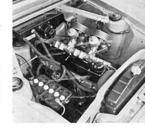
Kit includes high compression, aluminum alloy head, dual semidowndraft SU carbs, header system, oversize valves, tube push rods.
