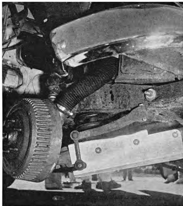
BELOW RIGHT. This '57 Ford has a heavy front stabilizer bar and oversize brakes. Special wide, finned drums have holes drilled through lining surface for better venting, receive ducted cool air.
