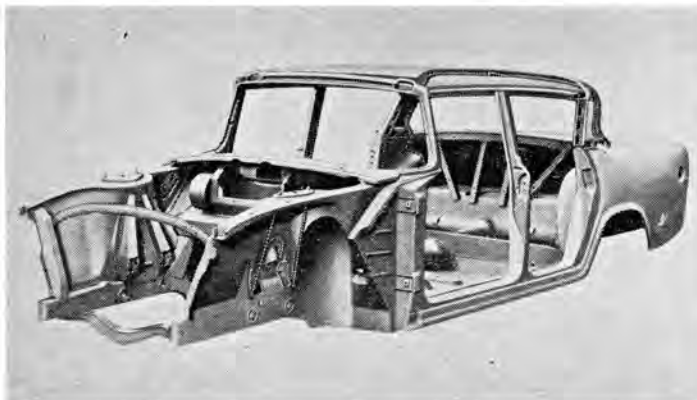
Unit construction of Rambler body and frame has nearly 9,000 welds which make the one-piece unit rattle-free. Mounting wells for the wide spaced front coil springs are stampings in fender panelling.
