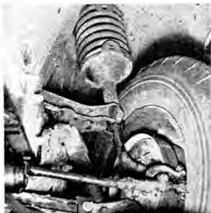
Front coil springs mount directly above spindle supports. Note wide cooling flange on brake drum which provides excellent stopping despite small nine-inch brakes.
