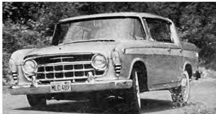
The Rebel is an agile car in city traffic and a cinch to maneuver into a parking place. Only the most violent cornering reveals the car has 58 percent of its weight up front.
