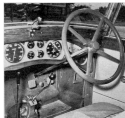
Interior is simple, with accelerator pedal located between clutch and brake. The four speed crash box has fairly close ratios.
