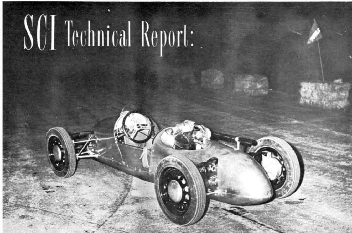
Fiat hubcaps are clue to suspension's ancestry. Jordan took two Topolinos—one front end from each—as his starting point and ended up with this very attractively turned out Formula III contender.
