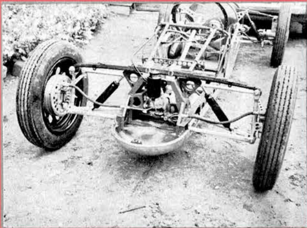
Slanted shocks lose out on leverage, but it definitely eases their installation. It's the only sensible way to install them on this narrow frame.
