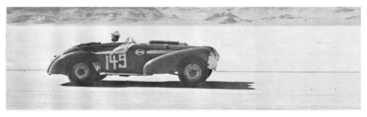
And that's the way it shouldn't be done. This Allard has gobs of brute power, but poor aerodynamics. Grille opening has been partially taped; but tremendous horsepower is required to overcome drag of the windscreen and the suction areas.
