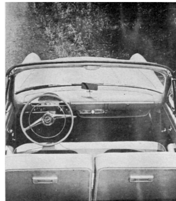
Instruments are grouped before the driver, and there is plenty of room. A power operated top is an option.
