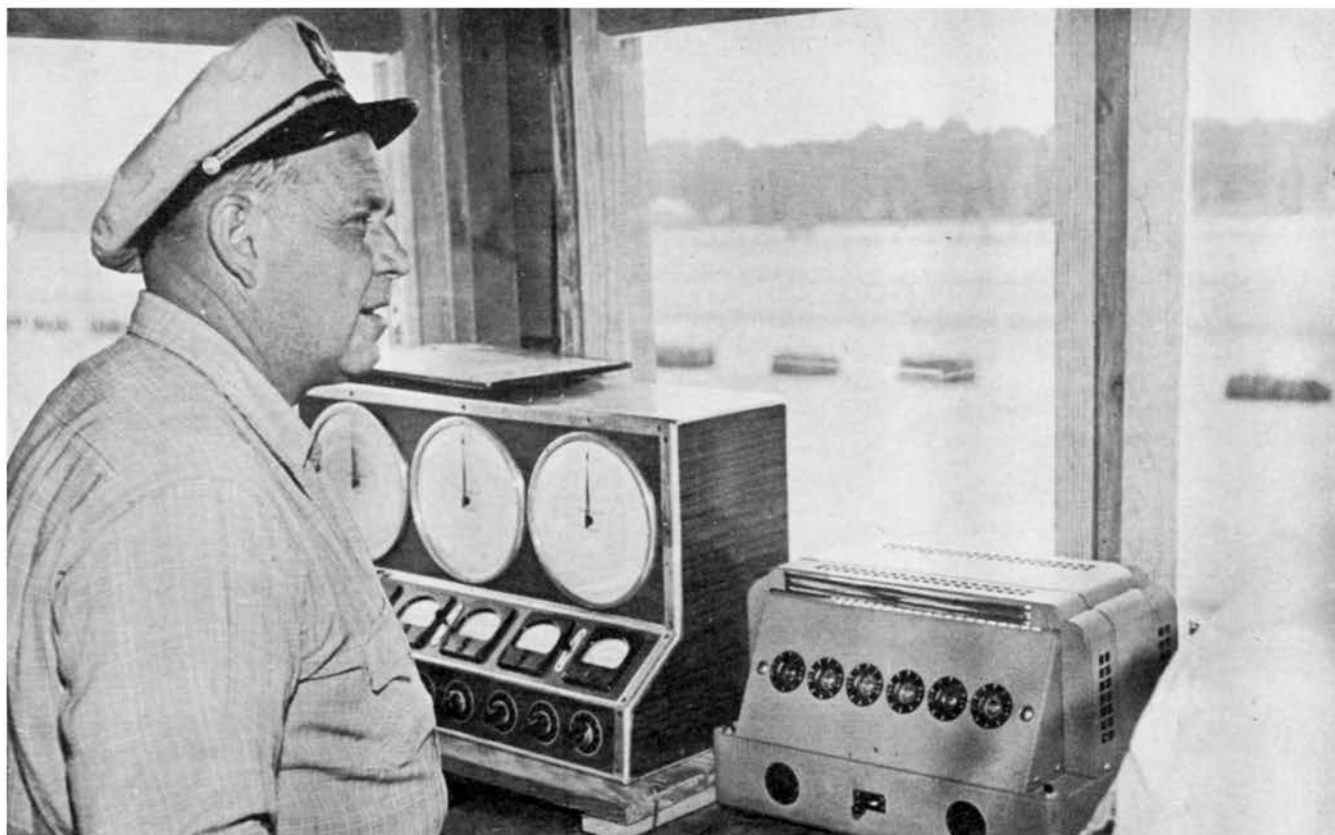
J. Otto Crocker, grand old man of timing with clock unit and the glow-tube electronic timer, accuracy attested to by Bureau of Standards to milliseconds.
