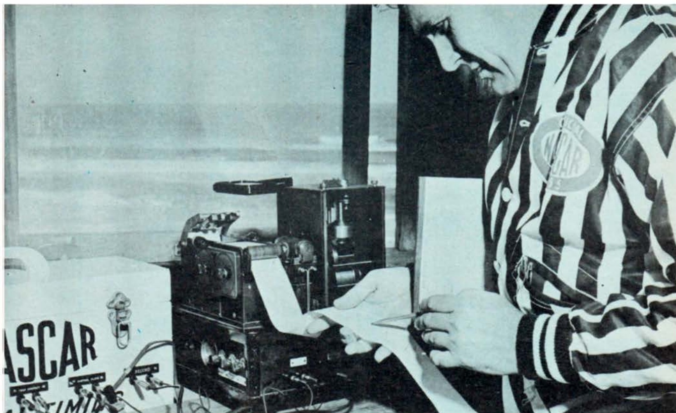
When tires pass over pneumatic hoses, elaborate mechanism inside NASCAR tower records the times of day at both ends. Hours, minutes and seconds are computed—mathematically—then are converted into mph—to nearest thousandth. (Oh!)
