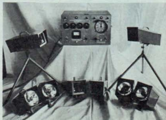
Top speed/elapsed time Chrondek unit, similar to Bonneville's, is extremely accurate and available.
