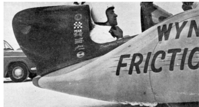
BELOW: The fastest U.S.-built car ever run was the Kenz-Leslie Streamliner, built by Bill Kenz, driven by Roy Leslie. Powered by three flat-head Fords, the car turned 270.473 one way; 266.204 average.
