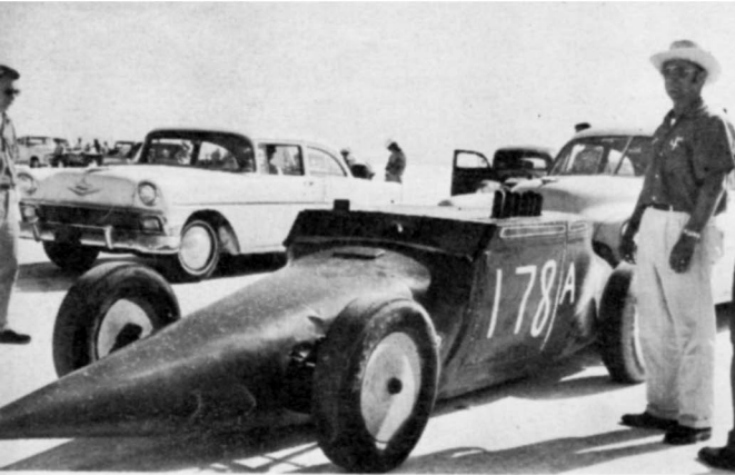
Coventry would probably look on this with mixed emotions. Veteran competition coupe took class A record at 125.596 with Jaguar engine using five pistons to bring displacement under 183 inches. #6 cylinder was blanked off but piston remained.
