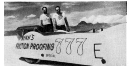
Here are Wynn's Friction Proofing distributors Bill Kenz and Roy Leslie, with their Streamliner, just before the record-making run. Two engines drive the front wheels, and the third engine, separately mounted, drives the rear wheels. Each engine has a displacement of 304 cubic in. for a total displacement of 912".
