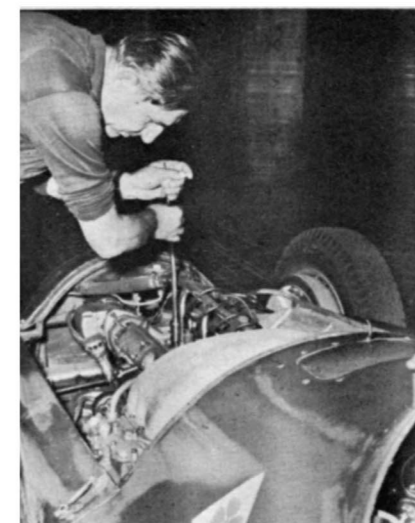
Zanardi, Alfa-Romeo's famous racing mechanic, finds plugs accessible on this otherwise complicated straight 8. Early models had one mag under exhausts.
