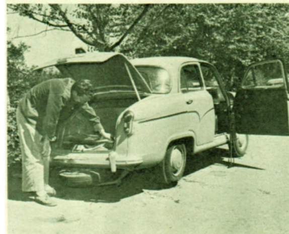
Editor Christy jacks up both wheels from one side jacking point. Spare tire tray is lowered by a spinner. Trunk space is more than adequate for a small car.
