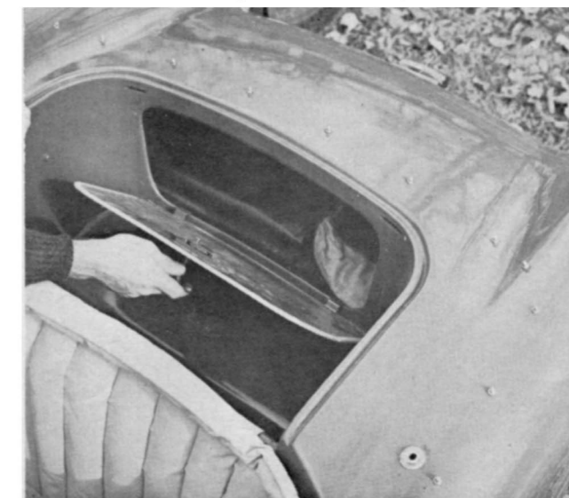
Jump seat will hold small child, but an adult will not fit in. Removing back of jump seat reveals huge storage compartment, holds roof. If edges are trimmed, spare will fit in, too.
