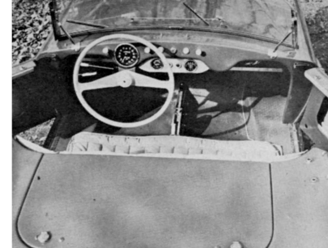
Instruments include speedometer calibrated to 120 mph, fuel gauge, ammeter. Reinforcing struts at edges of windshield are very practical. Gate-type gear shift splits cockpit. Jump seat/storage compartment deck pivots upward from seatback.
