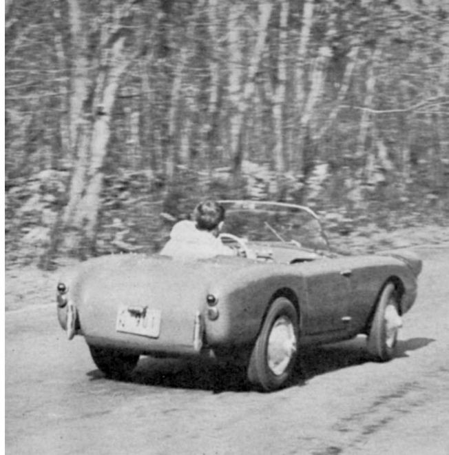
We forced the Berkeley sideways by cutting wheel, hitting brakes; no matter how rough we were, wheel correction and power brought tail in line. We were never in serious trouble.
