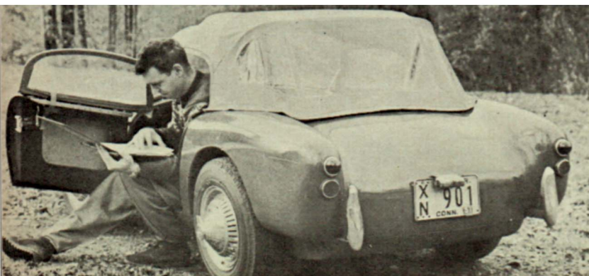
One of the sit-down-first-then-put-the-legs-in variety. Berkeley has a good finish, plenty of glass area, and independent rear suspension.
