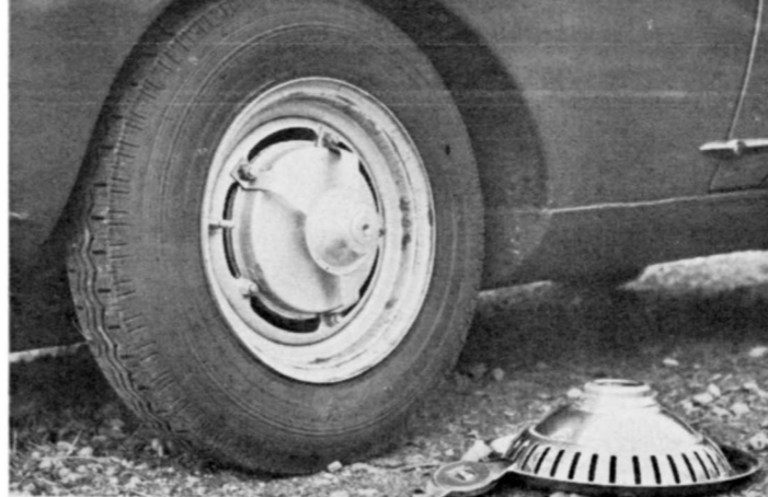
Seven inch brake drum is more than adequate for 760 pound car. Chrome hub is slitted for cooling air, and is held on by knock-off hub.
