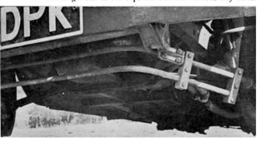
Another stability assist are these trailing radius rods that link the back axle to the side members. These rods control rear-axle dance, common to Anglias when cornering.
