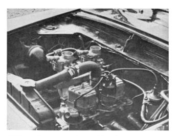
Willment Power Master head, with Rolls-fashion ohiv, is cast in aluminum alloy. Ribbed rocker boxes are antiresonant and minimize mechanical noise. The fourbranch-exhaust seen here is not a part of the Willment kit.
