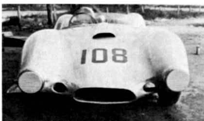
Alloy body was made by Lister's body builders. There is a strong resemblance around the air intake, although the Sadler's headlights are moved well forward.
