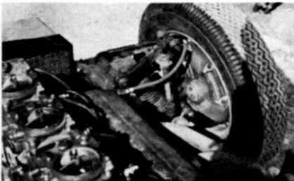
Front suspension incorporates Girling disc brakes and Armstrong spring-shock units. Modified Vauxhall anti-roll bar is shackled to the upper wishbone.
