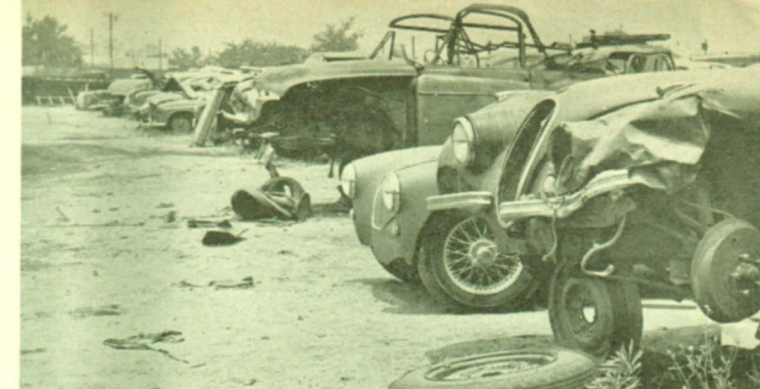
This Jaguar, hit from the left-front, makes purchases of front suspension parts a very risky business.
