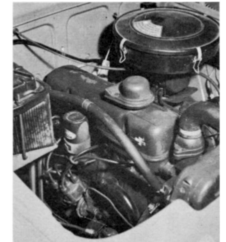
Unstressed, oversquare 1.5-ohv engine doesn't scream, should last a long time.
