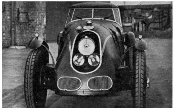
The Chrysler-A.E.C., with diesel bus engine, that did the last 6 of 24 hours with one of chassis side members broken in two.
