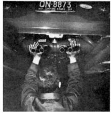
Place new muffler under car and insert lower pipes slightly. Then lift and place upper flanges over studs.
