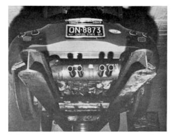
Cinch down the flange nuts and tighten the muffler clamps over lower pipes. Then replace the splash shield and you're in business. The total job shouldn't take over an hour or so.
