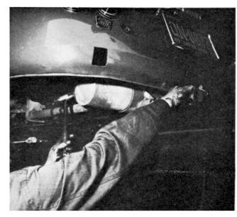
Using a rubber mallet, tap the old muffler gently at either end until it drops free from both pipes and upper flange studs. Be careful not to damage or burr the studs in any way.
