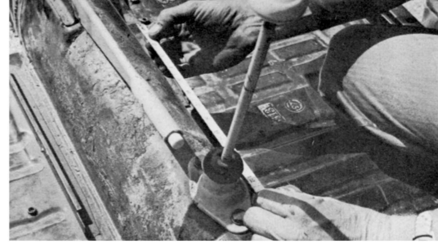
With the driver's seat moved back, you will want to move the shift lever, too. Buckland decided on twelve inches aft, but didn't shorten the lever as many stock VW owners do.
