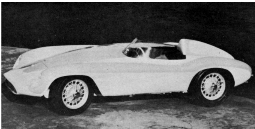
Finished Beetle (not Ted's) features Dayton wire wheels, filled in front fender holes, rigid tonneau cover, and modified engine cover using Porsche grille for air intake. Last major step is to chop 2½ inches from top of cooling shroud. Shorten oil cooler, too, and remove shroud's internal baffles.
