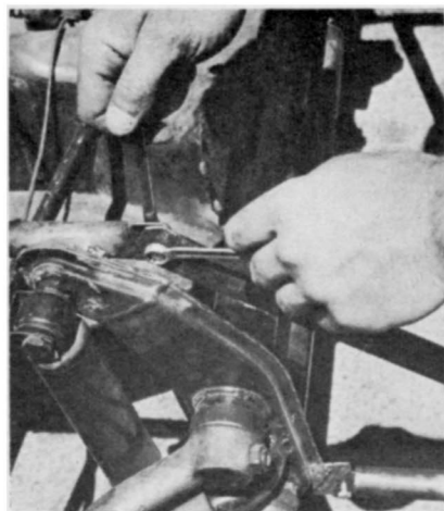
The forward auxiliary framework must be removable so that the body may be slipped on. The upper portion bolts to the front shock absorber mount; the lower to a flange welded to the frame.
