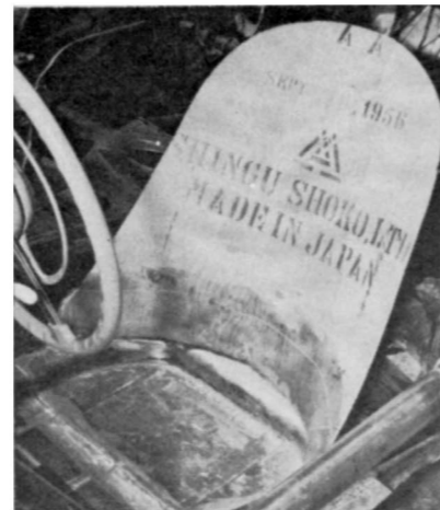
In the Devin-VW, the driver sits lower and further back than before. Buckland laminated his "imported" seat-back to the floor with cloth and resin. Remove seat rails, make seat cushion to fit.
