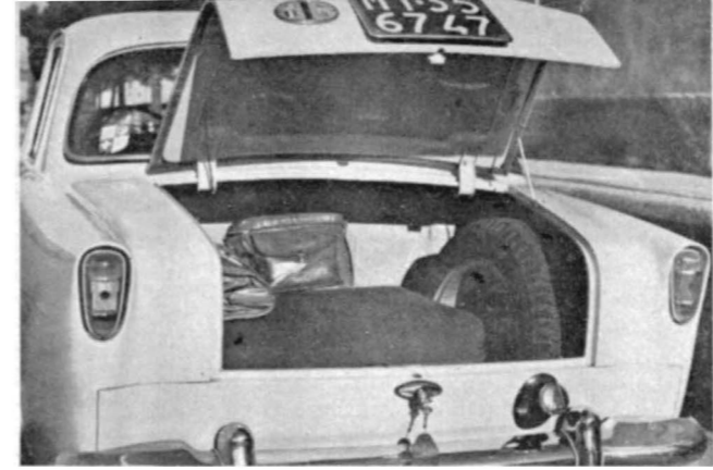
Plenty of room for passengers and their luggage. Trunk opens upwards, exposes Pirelli-fitted spare, tools and space.
